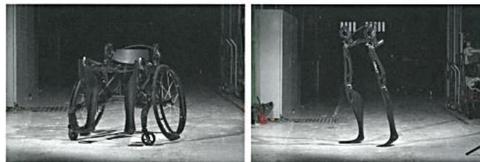
A carbon fibre composite wheelchair combined with an exoskeleton to assist a person getting up, prototype by Uchida (2016) © Uchida
